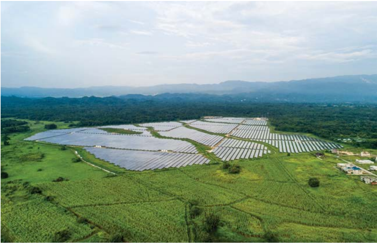
A 37-MW solar photovoltaic power generation plant at Paradise Park in Westmoreland, Jamaica. The plant is expected to contribute 74,000 MWh to the national electricity grid annually. It will displace about 107,000 barrels of fuel annually, while preventing over 48,000 tonnes of CO2 emissions.
