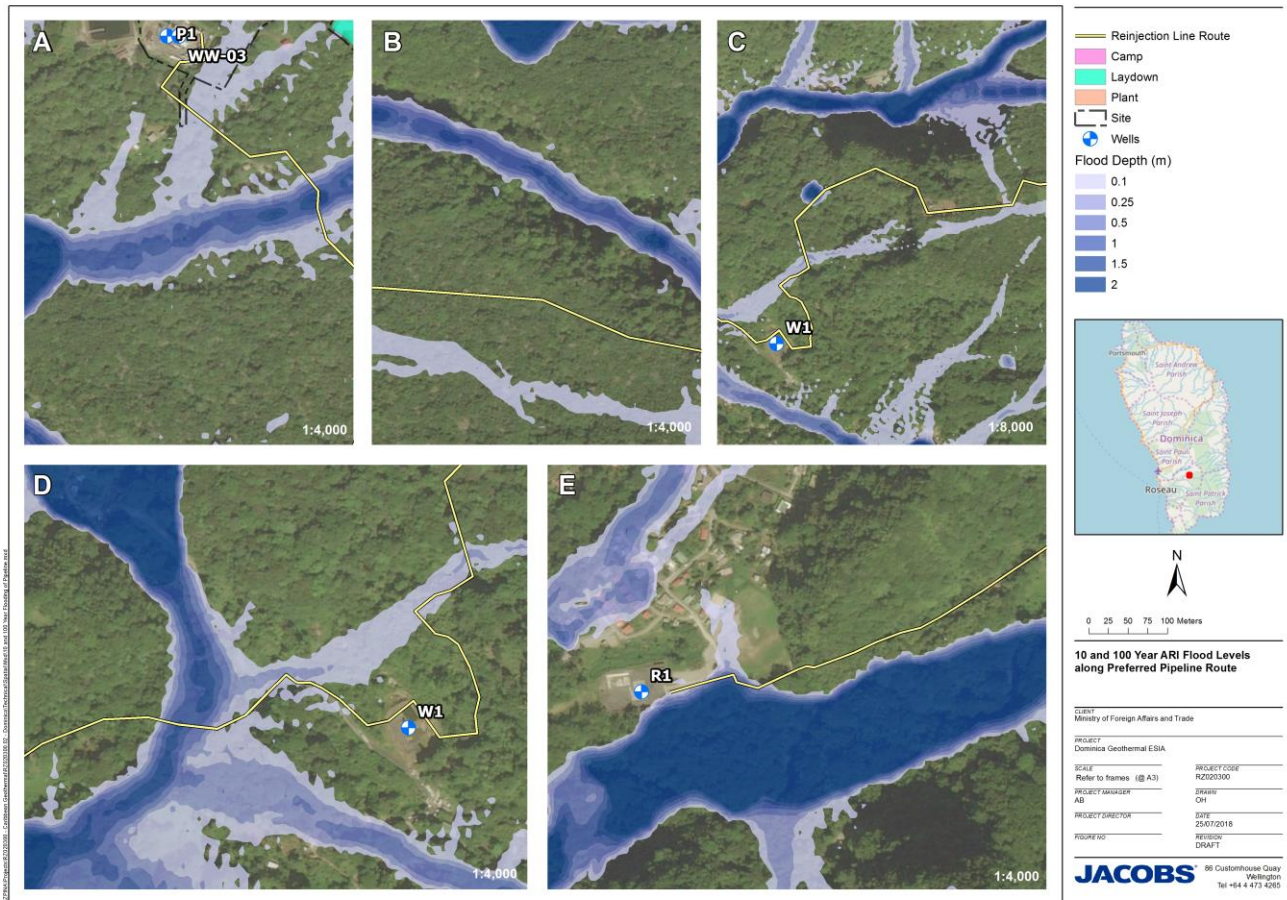
Figure 7.3 : 100 yr ARI 12 hour flood water levels and the at risk areas of preferred pipeline route.
