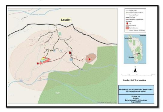
The proposed reinjection site is located at the west of the community. The soil was assessed to identify soil type and sub-surface water absorption capacity at 4ft at the proposed site identified for reinjection of the geothermal wastewater. Two holes were dug at a depth of about four feet and filled with water up to a level of one foot to identify the speed at which water is absorbed to determine subsurface characteristics.
