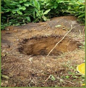
Soil samples were taken at three sites to include the proposed power plant where the pipeline begins, one along the proposed pipeline and one near the point of reinjection, to establish a baseline of the contaminant levels at the points of sampling. Samples were analyzed for the following parameters: arsenic, mercury, lead and salinity.
