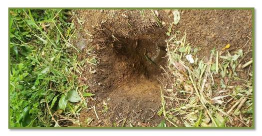
The two holes were filled with water up to one foot and allowed to percolate over a period of ninety minutes. Water in hole 1 (one) dropped about three inches and hole two dropped about five inches over that period.
